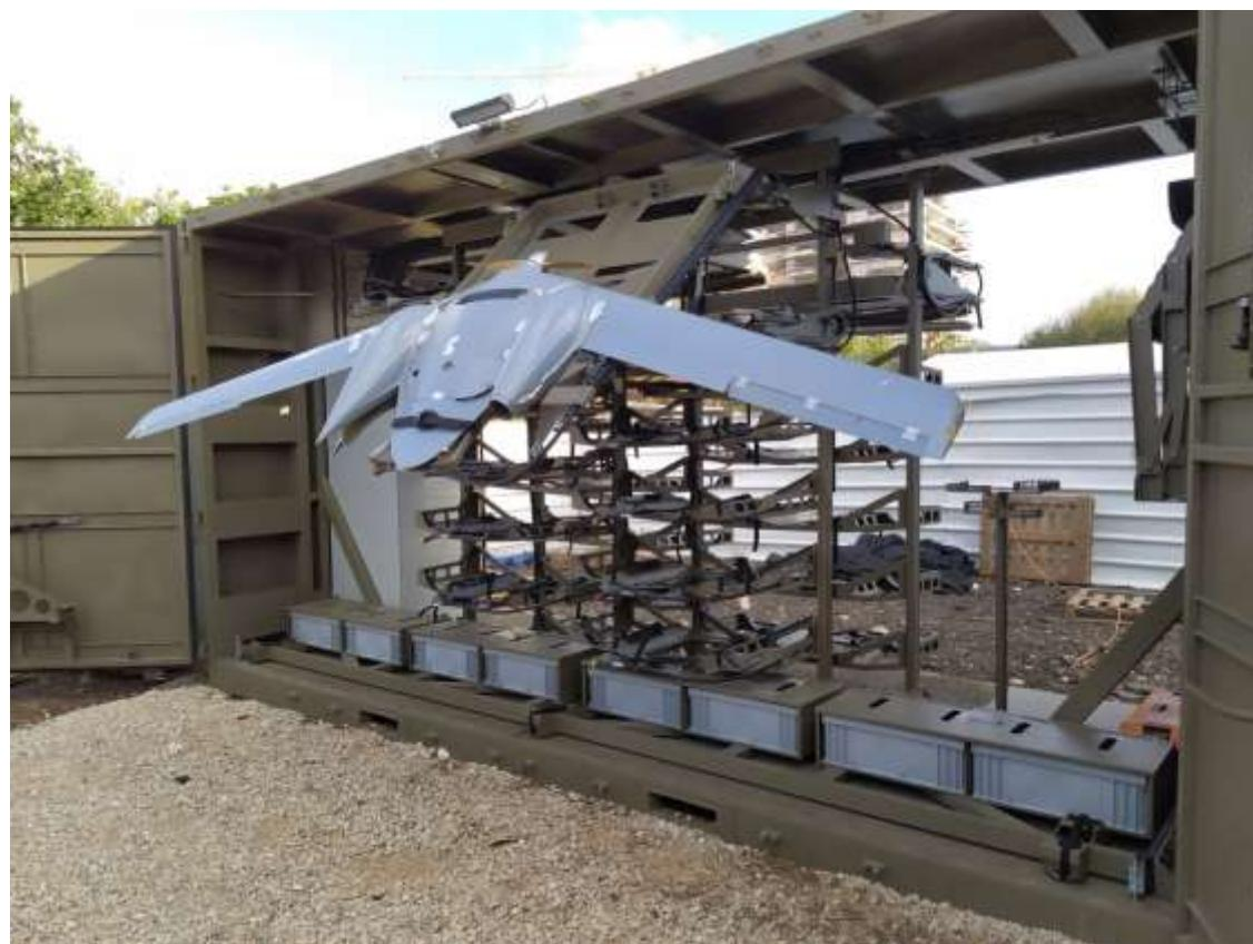
**The UAV Container** intended for transportation of Unmanned Air Vehicles.
